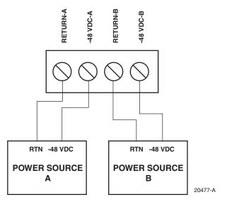
Figure 2-3. Four-Pin Power Plug Wiring Diagram
